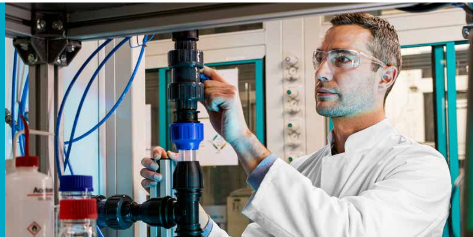
+ Chemical Engineer Dr. Peter Schulze is adjusting the air flow at the pilot plant for carbon dioxide direct air capture (CODA project).
