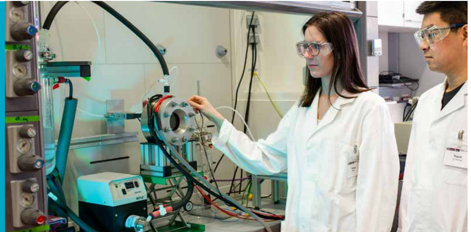
+ IMPRS doctoral candidate Tamara Miličić and her Master student Thanh Hoang Vu are performing experiments on the proton exchange membrane water electrolysis test bench.
