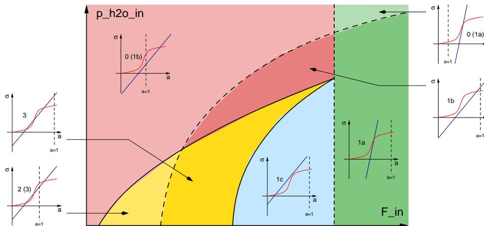
**Fig.6:** Qualitative two-parameter bifurcation diagram for a simplified PEM fuel cell model in resistostatic operation mode, showing regions of three to zero solutions.
