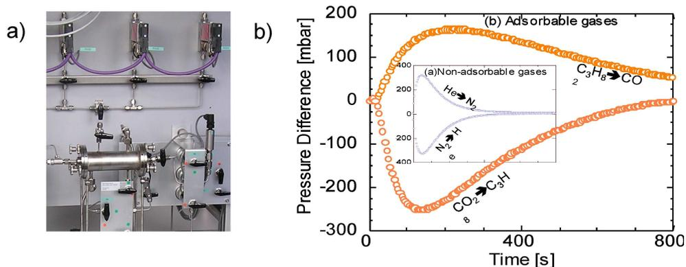
**Fig. 11:** **a)** Experimental setup (modified Wicke Kallenbach cell); **b)** Obtained pressure response curves for two transient exchange experiments using a porous glass membrane.
