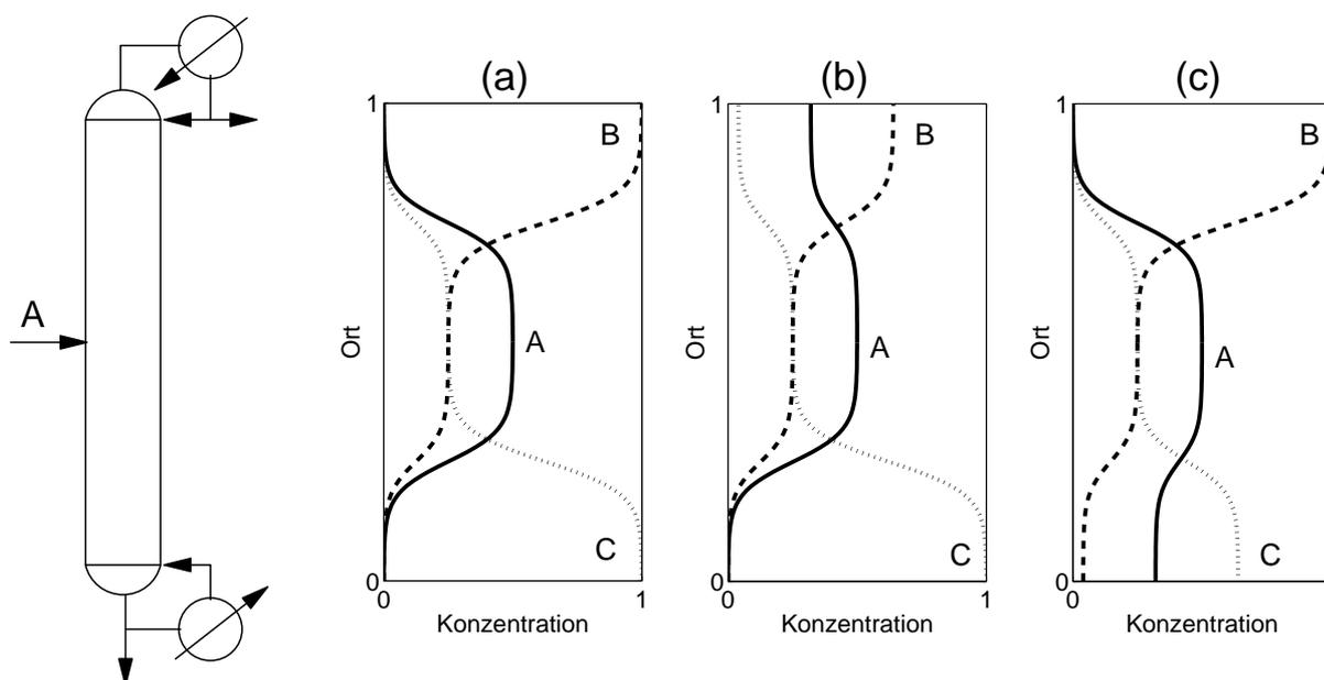
**Fig. 2:** Characteristic steady state concentration profiles in a reactive distillation column with a chemical reaction of type  $2A \rightleftharpoons B + C$  in the liquid phase. (a) Reactant A has intermediate volatility. (b) Reactant A has highest volatility. (c) Reactant A has lowest volatility.
