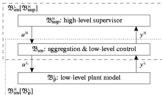
**Fig. 2:** Two-level control architecture
