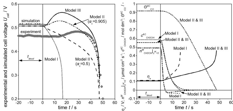
**Fig.5:** Dynamic simulation of DMFC showing impact of different electrode kinetics (Model I, II, III), especially the importance of accounting for adsorbed reaction intermediates on the anode ( $CO$  surface coverage  $\theta_{CO}^{AC}$ )
