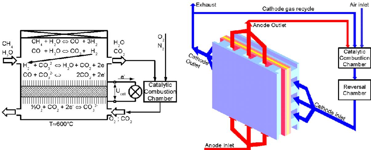
**Fig.7:** Schematic of MCFC with DIR (left), compartments and mass flows of the 2D MCFC model (right)
