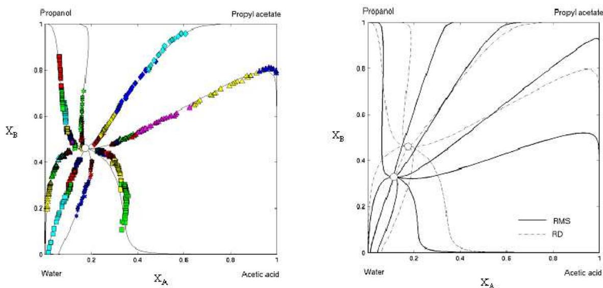
**Fig.3:** Residue curve maps for the synthesis reaction of propyl acetate ( $Da \rightarrow \infty$ ) (a) Experimental validation of reactive distillation RCM (b) Prediction of the reactive a-rheo-trope under the influence of porous polycarbonate membrane of pore size 50 nm.
