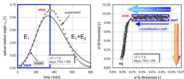
**Fig. 8:** Typical optical rotation angle curve (**left**) and trajectories (**right**) for reproducible batch experiments. Comparison (**left**) of the experimental  $\alpha$ -curve obtained by seeding with L-threonine ( $E_1$ ) crystals with simulations (Elsner et al., 2005a).
