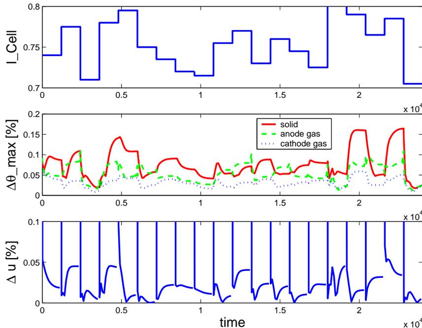
**Fig. 8:** Model reduction of a 2D MCFC model (Grötsch et al., 2005). Comparison between the reduced model's response to a randomly varying cell current and the reference model's response; top diagram: dimensionless cell current used as input signal for the models; middle diagram: maximal relative error of the temperatures in the stack; bottom diagram: maximum voltage error.
