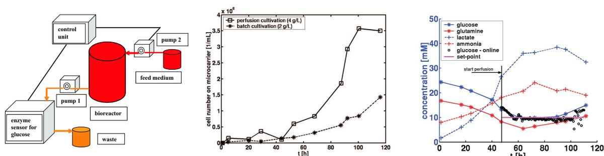
**Fig. 3:** Left: Scheme for closed-loop glucose control; middle: cell numbers on microcarriers during growth of MDCK cells in a 5L-stirred tank bioreactor (0-118 h). \* 2 g/L Cytodex 1 batch; □ 4 g/L Cytodex 1 with perfusion as shown left; right: Glucose on- and off-line data as well as lactate data for the perfusion cultivation as shown left.
