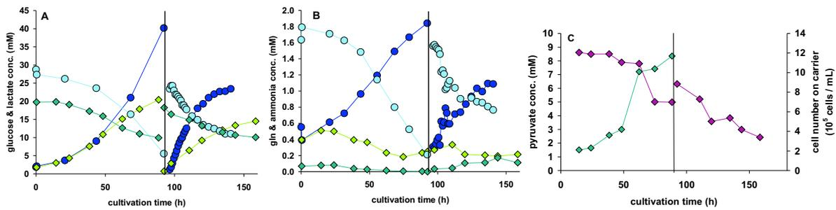
**Fig. 5:** Release & uptake of metabolites, cell numbers in gln-medium and pyr-medium during growth of MDCK cells in a 5L stirred tank bioreactor (0-93 h) and during influenza virus production (93-158 h, vertical line). (A) gln-medium: ● glucose, ● lactate; pyr-medium: ◆ glucose, ◆ lactate; (B) gln-medium: ● glutamine, ● ammonia; pyr-medium: ◆ glutamine, ◆ ammonia; (C) pyr-medium: ◆ pyruvate, ◆ cell number on carrier.
