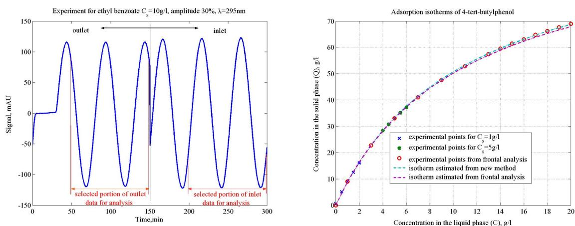
**Fig. 4:** (left) Example of periodic input and output data; (right) Determined adsorption isotherm of 4-tert-butylphenol (Ilić et al., 2005).
