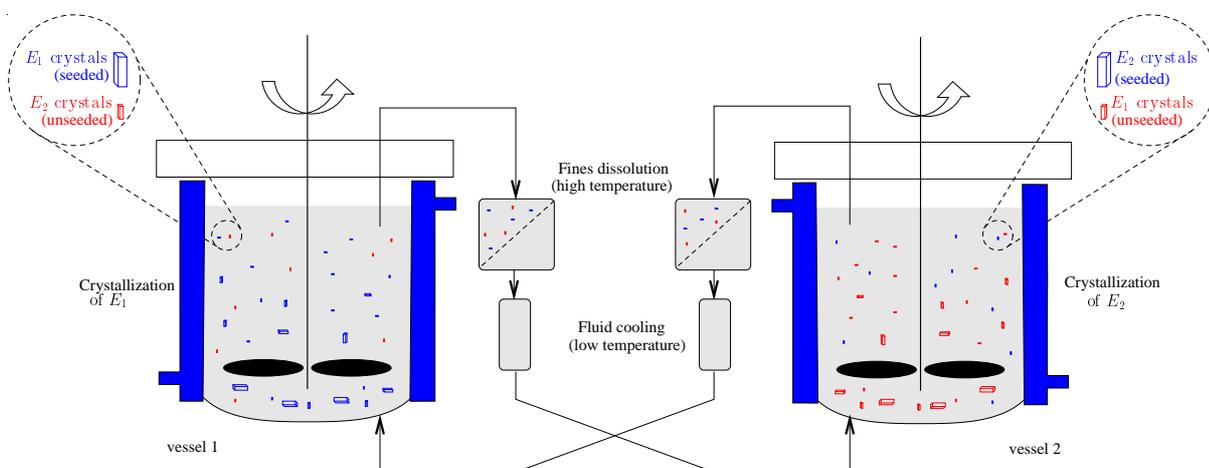
**Fig. 6:** Simultaneous batch-crystallisation.
