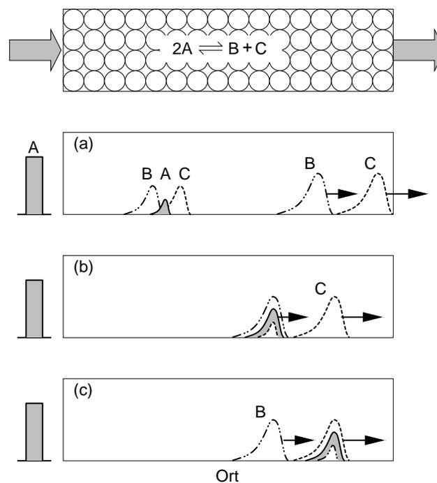
**Fig. 3:** Characteristic pulse patterns in a fixed bed chromatographic reactor with a chemical reaction of type  $2A \leftrightarrow B + C$  in the liquid phase. (a) Reactant A has intermediate adsorptivity. (b) Reactant A has highest adsorptivity. (c) Reactant A has lowest adsorptivity.
