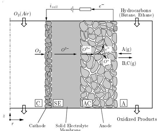
**Fig.10:** Schematic of electrochemical membrane reactor (EMR)
