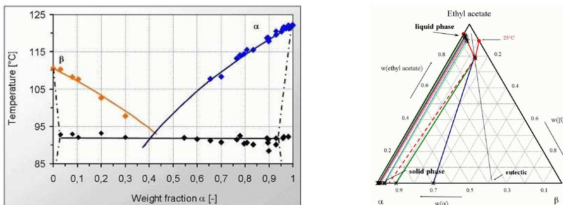
**Fig. 2:** (left) Melting point phase diagram of an isomeric system; (right) Solubility phase diagram of the  $\alpha$ - and  $\beta$ -isomers of the diastereomeric intermediate in ethyl acetate (Gedicke et al., 2005).
