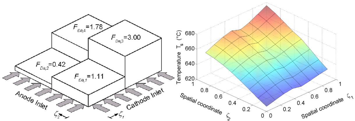
**Fig.8:** Optimal distribution of reforming catalyst in terms of relative catalyst density (left), resulting spatial temperature distribution (right).
