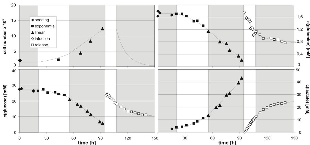
**Fig. 11:** Cell numbers (upper left) and concentration profiles of glutamine (upper right), glucose (lower left) and lactate (lower right) during the standardized vaccine production process. For MFA the process was divided into 5 characteristic stages, the seeding (0-20h), exponential (20-55h), linear (55-95h), infection (95-107.5) and virus release (107.5-150h) phase, denoted by gray and white shadings. The lines represent the results of the multiparameter regression analysis.
