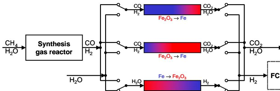
**Fig.13:** Conceptual design of periodically operated methane steam reformer system
