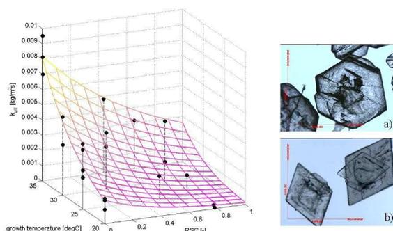
**Fig. 3:** (left) Effective growth rate constant  $k_{eff}$  versus growth temperature and the relative solvent composition RSC for growth of (S)-mandelic acid from aqueous solution; (right) Microscopic images of (S)-mandelic acid crystals obtained a) in absence and b) in presence of the counter enantiomer in solution.
