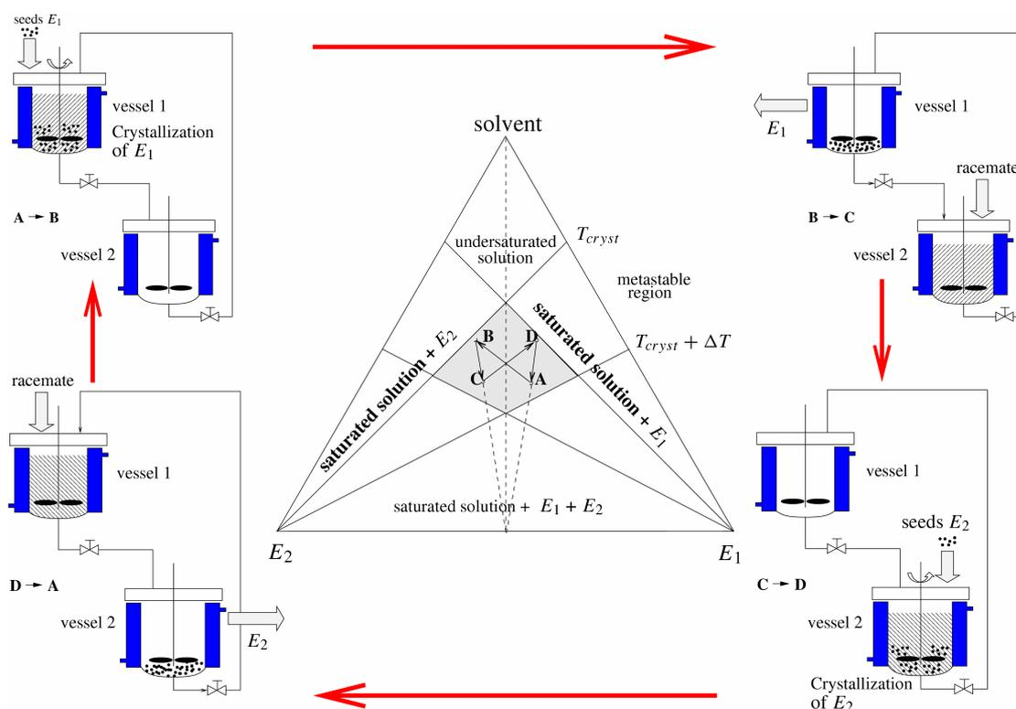
**Fig. 5:** Cyclic batch process for enantiomer separation.
