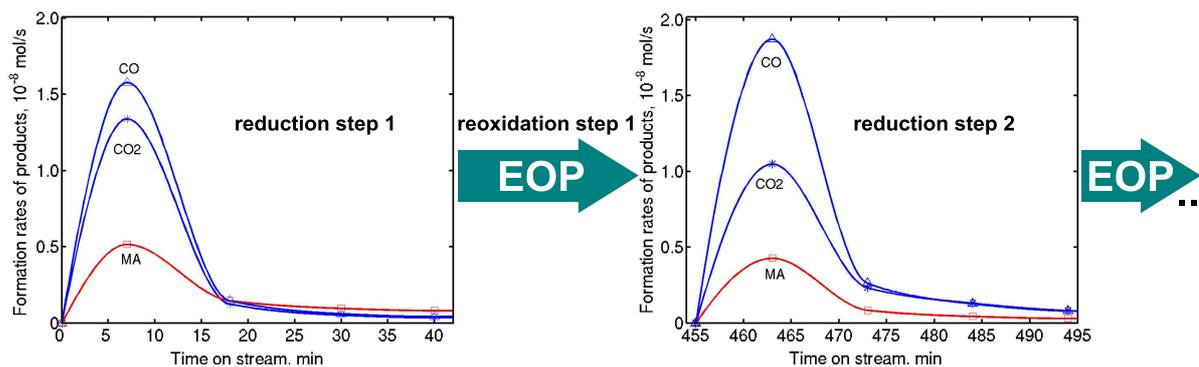
**Fig.11:** Experimental results from EMR redox cycle operation (production of maleic anhydride, MA, and intermediary catalyst reoxidation by electrochemical oxygen pumping, EOP)
