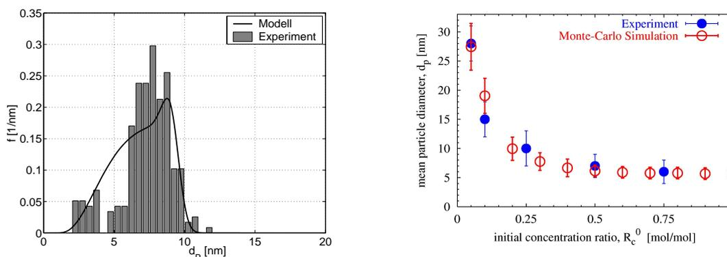
Fig.15: Comparison between experimental and simulation data for barium sulfate precipitation in microemulsion. Left: Population balance model; Right: Monte-Carlo simulation for variation of initial concentration ratio.
