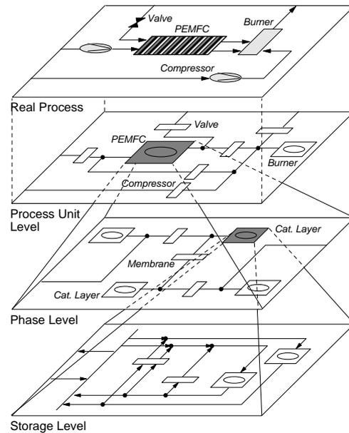
**Fig.12:** Levels of process structuring for a fuel cell system.
