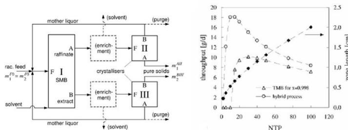
**Fig. 12:** (left) Example for two coupled separation processes. A racemic feed is partially resolved by SMB-chromatography and then split into the pure enantiomers by subsequent enantioselective crystallization. (right) Numerical simulation for mandelic acid enantiomers reveals the possibility of increased throughput of the coupled process (open circles) compared to the stand alone chromatographic separation (triangles). (Kasperleit et al., 2005).
