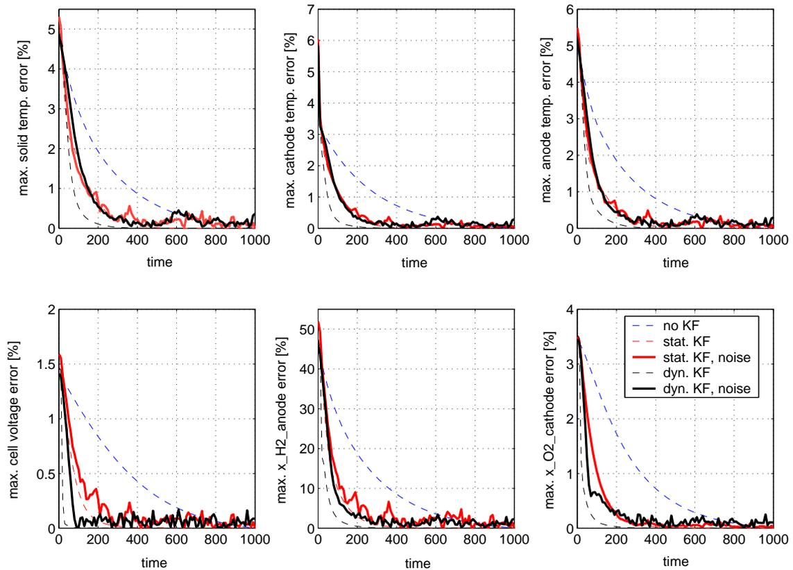
**Fig. 9:** Convergence behaviour of a static and a dynamic Kalman filter for the HotModule (Grötsch et al., 2005); simulation results with artificial noise are used as virtual measurement data.
