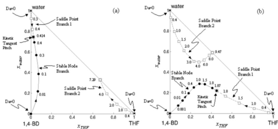
**Fig.2:** Potential singular point curves (PSPS) and bifurcation behaviour for system: 1,4-BD  $\rightarrow$  THF + Water ( $p = 5$  atm). (a) Reactive distillation (b) Reactive membrane separation with Knudsen diffusivities.
