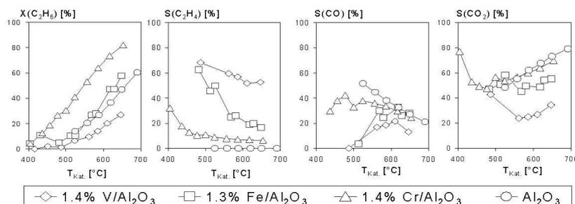
**Fig. 5:** Conversion (X) and selectivity (S) for different transition metal components as a function of temperature. Conditions: 0.7 % ethane in air, GHSV =  $38000 \text{ h}^{-1}$  (Klose et al., 2004a, 2004b).
