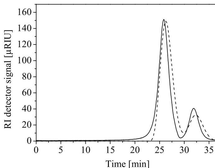
**Fig. 4:** Experimental (solid line) and simulated elution profile (dashed line) for MF hydrolysis taken from (Vu et al., 2005).
