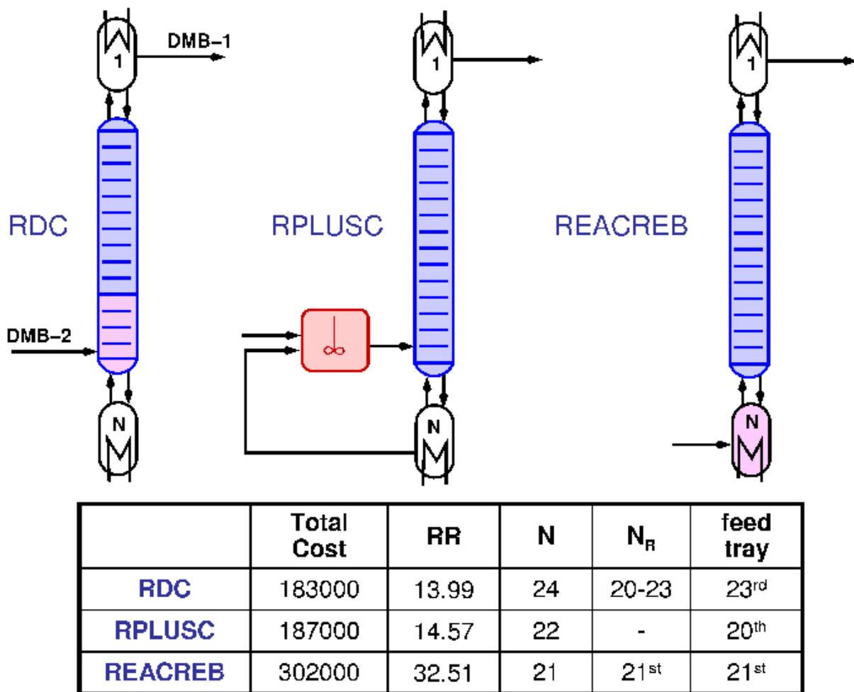
**Fig. 6:** Production of DMB-1 by isomerisation from DMB-2 by combined reaction distillation processes. Process candidates and results from a local MINLP optimization.
