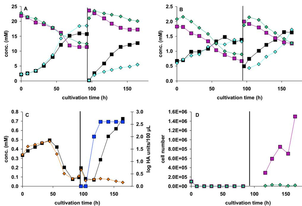
**Fig. 6:** Release & uptake of metabolites, cell numbers and virus titer in infected and mock-infected roller bottle during growth of MDCK cells (0-96 h) and during influenza virus production (96-165 h, vertical line). (A) infected: ■ glucose, ■ lactate; mock-infected: ◆ glucose, ◆ lactate; (B) infected: ■ glutamine, ■ ammonia; mock-infected: ◆ glutamine, ◆ ammonia; (C) infected: ■ HA-value, ■ glutamate; mock-infected: ◆ glutamate; (D) cell number in supernatant: ■ infected, ◆ mock-infected.
