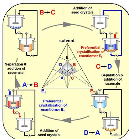
**Fig. 7:** Principle of the preferential crystallization and a possible cyclic operation mode.
