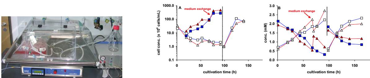
**Fig. 2:** Left: Wave bioreactor with a 1L wv cell bag; middle & right: cell numbers, release & uptake of metabolites in serum containing medium during growth of MDCK cells in a wave reactor (0-99 h) and during equine influenza virus production (99-164 h, dashed vertical line). ■ 2 g/L Cytodex 1; ▲ 4 g/L Cytodex 1 (arrow indicates medium exchange of 500 mL medium). For (A): cells on microcarriers: ■; ▲, cells in supernatant: □; △. For (B): glutamine: ■; ▲; ammonia: □; △.
