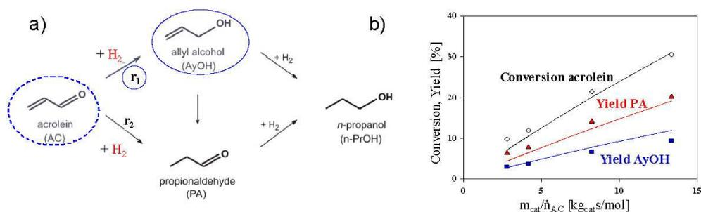
**Fig. 6:** a) Reaction network of the hydrogenation of acrolein to allyl alcohol; b) Conversion and yield as a function of space velocity ( $\text{Ag}/\text{SiO}_2$  catalyst) (Hamel et al., 2005).
