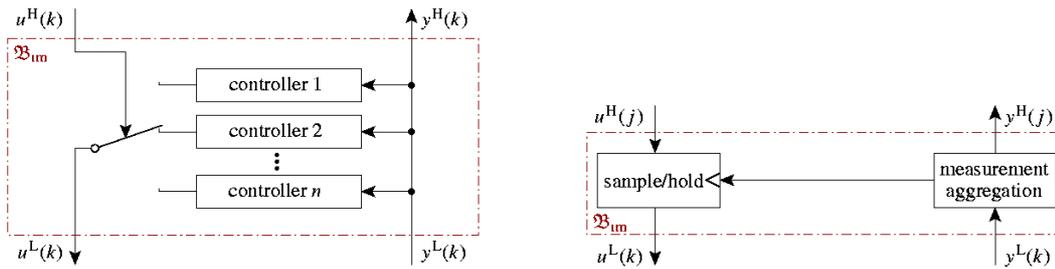
**Fig. 3:** Intermediate layers implementing switching between low-level controllers (left) and measurement aggregation in time and signal space (right).
