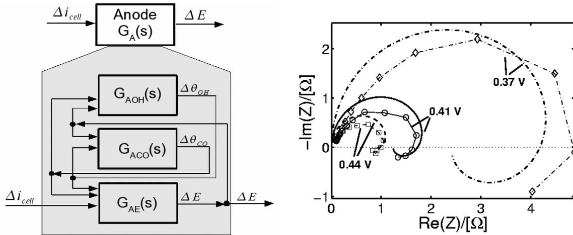
**Fig.4:** Block diagram of DMFC anode model (left), and simulated and experimental EIS data (right)
