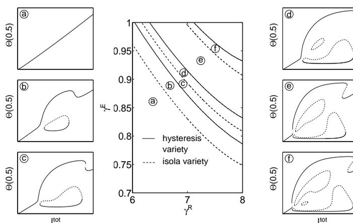
**Fig.9:** Bifurcation analysis of high-temp. fuel cell model; Center: Co-dimension 1 singularities in the parameter plane spanned by Arrhenius numbers of electrochemical reaction and the electrolyte's electrical conductivity, respectively. Surrounding diagrams: Continuation of steady-state solutions using total cell current as bifurcation parameter.
