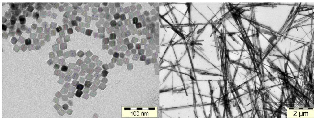
**Fig.14:** TEM pictures of crystalline barium sulfate (left) and calcium carbonate needle-like nanoparticles (right).
