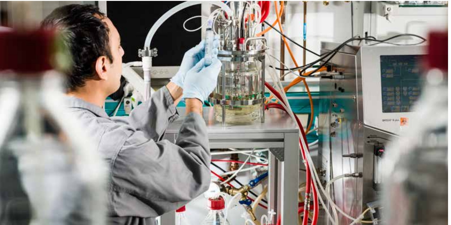
+ For the optimization of production processes using mammalian cells one aim is to increase the cell concentration in bioreactors. Such high cell density cultivations require novel techniques to continuously provide nutrients for cell growth. Here, Ph.D. candidate Daniel Vázquez Ramírez is testing different perfusion systems such as the depicted alternating tangential flow (ATF) system.
