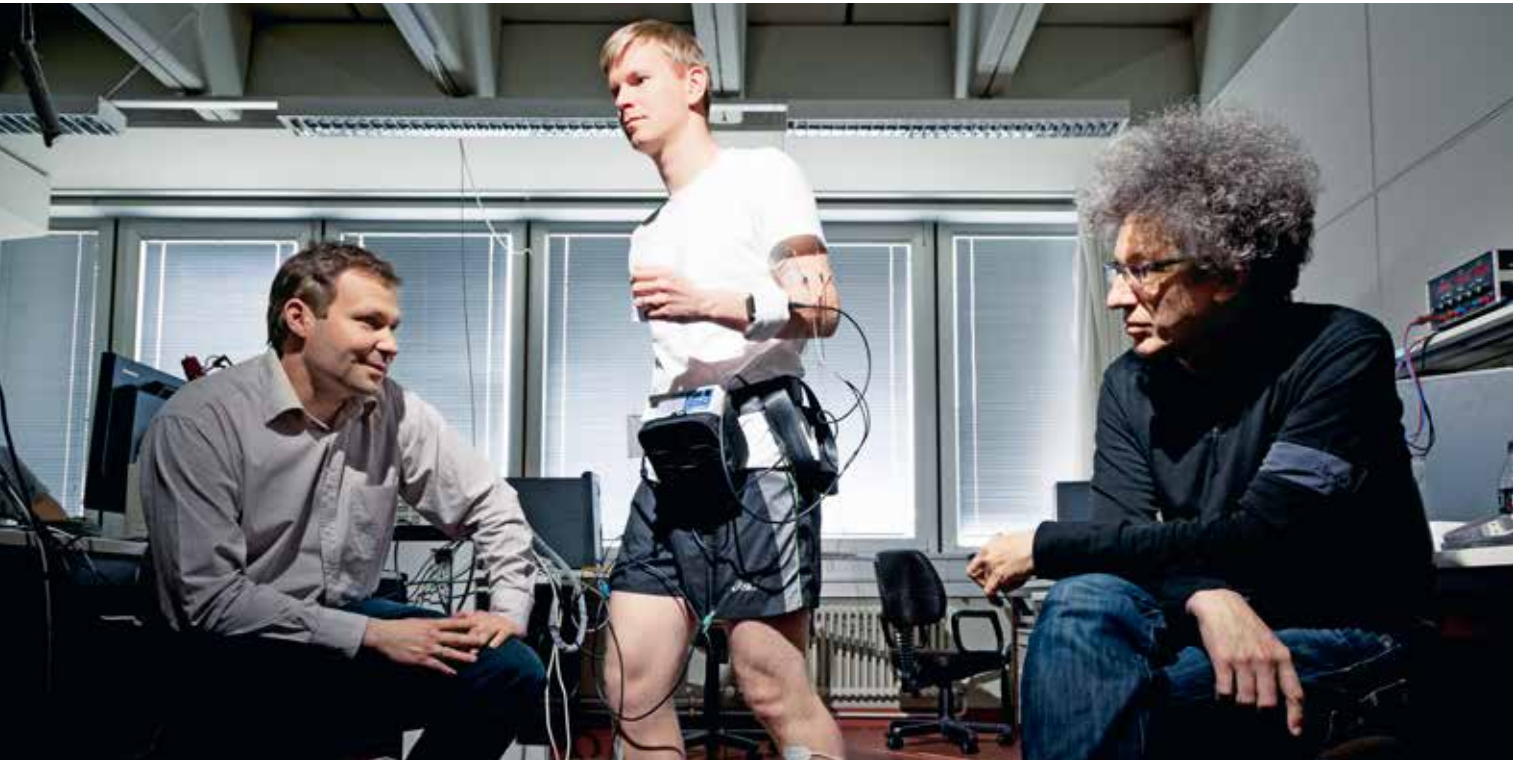
+ Testing an adaptive drop-foot stimulator intended for stroke patients. The underlying control concept is based on ideas from Iterative Learning Control (ILC). Left and right: Dr. Thomas Schauer (TU Berlin), Prof. Dr.-Ing. Jörg Raisch. (Healthy) test person in the middle: former Ph.D. student Thomas Brunsch.
