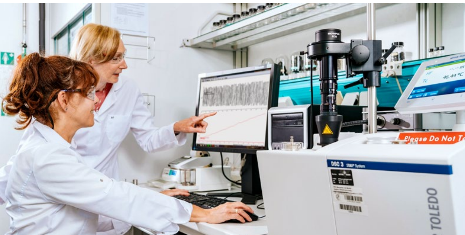
+ Jacqueline Kaufmann and Heike Lorenz are discussing the results of thermo-analytical studies of a fine chemical. To deeper understand its phase behavior temperature-modulated differential scanning calorimetry (DSC/TMDSC) and combined DSC-microscopy are used.
