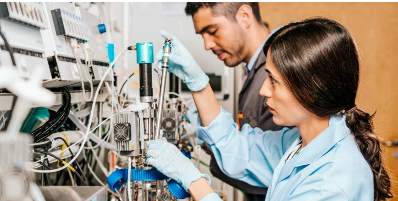
+ Gwendal Gränicher and Julia Coronel de Lima Lagos are introducing sensors into small scale bioreactors in preparation for a new experiment.
