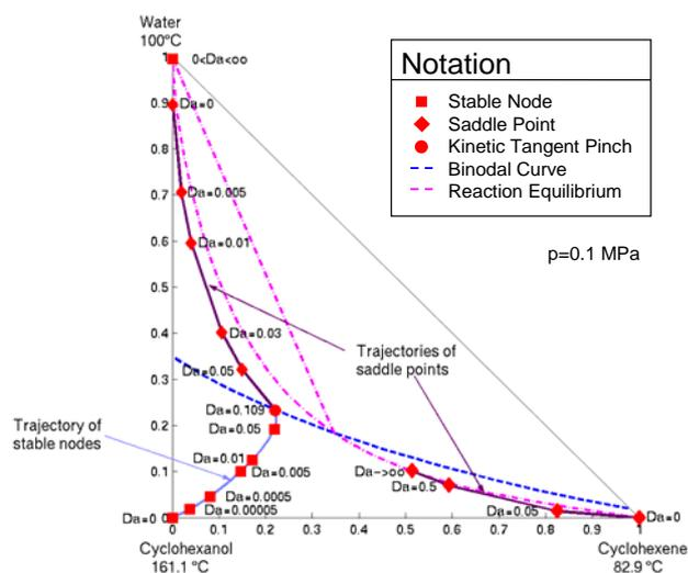
**Fig. 23:** Bifurcation diagram of singular point in dependence on the Damköhler number [5].
