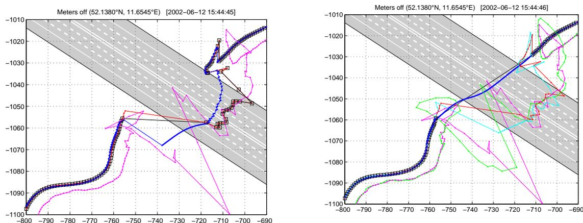
Original situation: GPS multipath reflections around the bridge confuse the controller.
