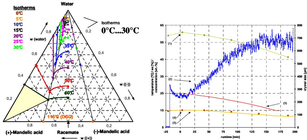
**Fig. 55** Left: Ternary solubility phase diagram of the mandelic acid enantiomers in water [10 – 12]. Right: Batch crystallization experiment for purification of an asymmetric mixture of mandelic acid in water ((1) enantiomeric excess of solution (ee) , (2) median crystal size (FBRM), (3) temperature profile in the crystallizer, (4) solute concentration (offline, density measurements), (5) solute concentration (inline, acoustically determined)) [13].
