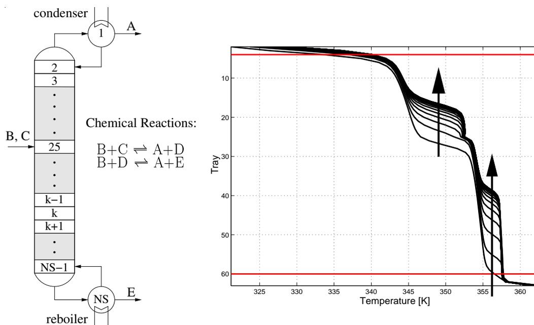
**Fig. 16:** Traveling temperature fronts in an industrial reactive distillation column after a step change of the heat duty.
