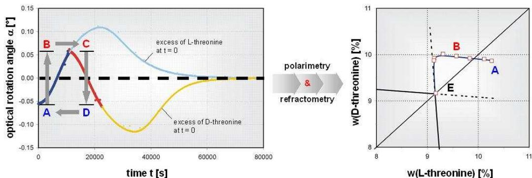
**Fig. 57:** Left: Polarimetric signal for the resolution of both enantiomers. Right: Phase diagram for the preferential crystallization process with an excess of L-threonine at the beginning (point A) [14].
