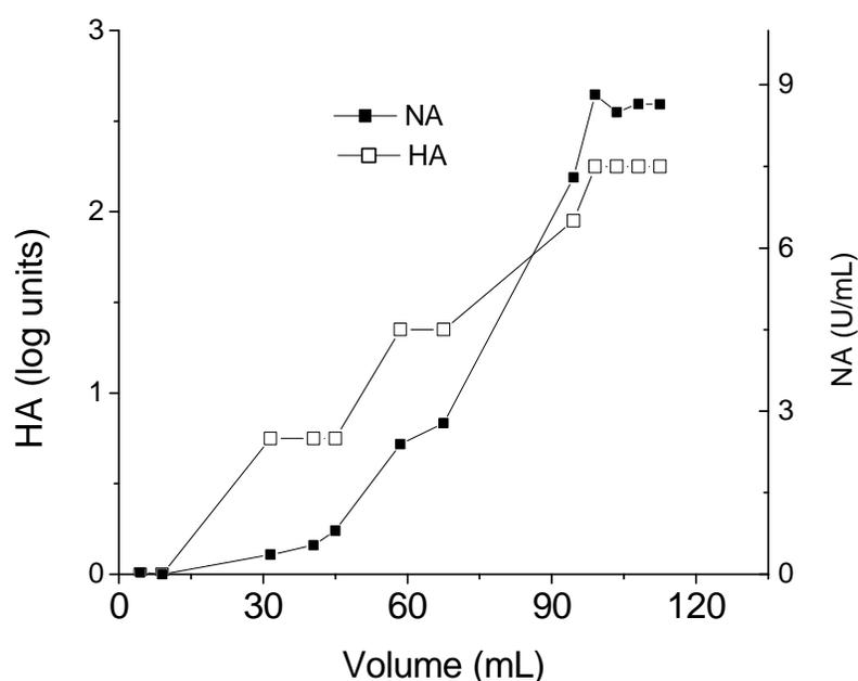
**Fig. 74:** Breakthrough curve of inactivated equine influenza virus showing HA and NA activities from affinity chromatography in a packed bed.  $V$  and  $C$  denote volume and concentration of the effluent where as  $C_0$  and  $V_C$  are the feed concentration and column volume, respectively.
