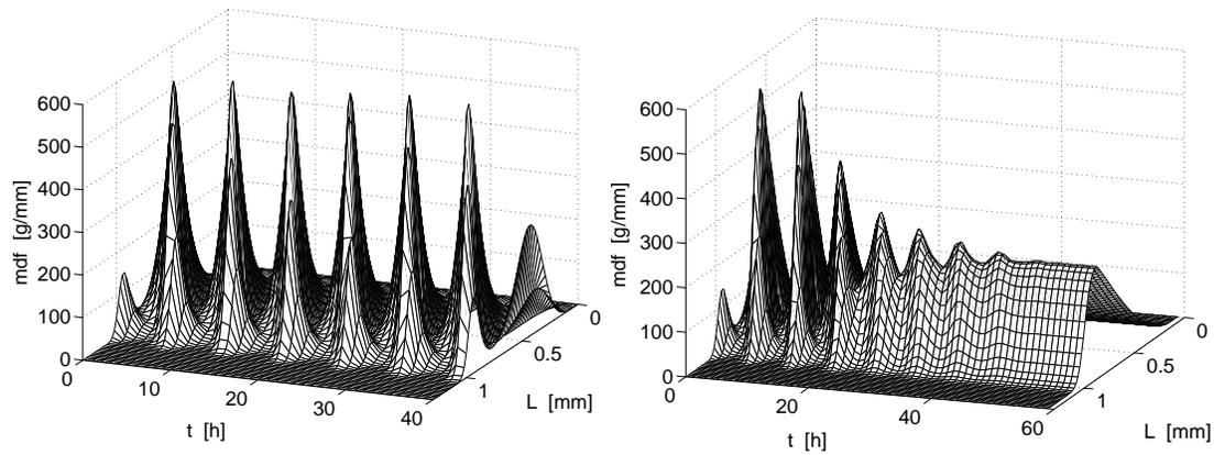
**Fig. 42:** Oscillating CSD without control (left); control switched on at  $t_0 = 10h$  (right).
