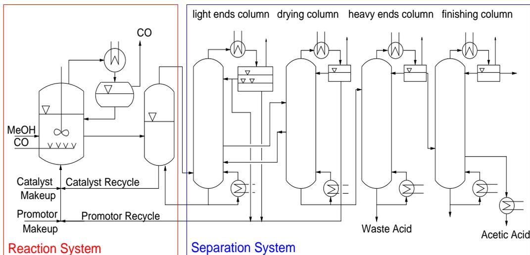
**Fig. 20:** Simplified flowsheet of an industrial plant for the production of acetic acid.
