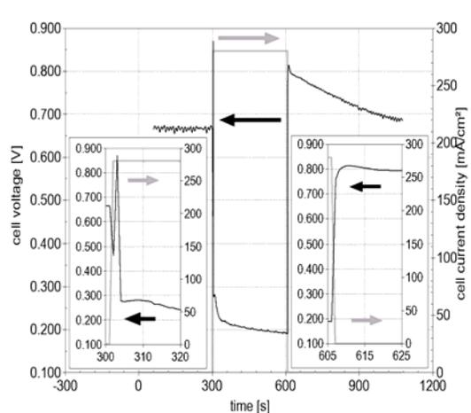
**Fig. 31:** Cell voltage response to a pulse change of the current density obtained from a miniplant experiment [20].
