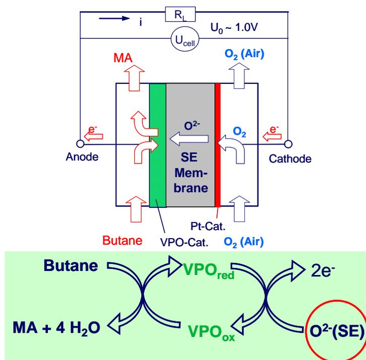
**Fig. 36:** Working principle of electrochemical membrane reactor for partial oxidation of butane to malenic acid (MA) [28].
