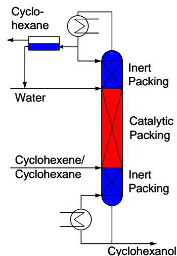
**Fig. 24:** Flow scheme of proposed reactive distillation process for cyclohexanol synthesis [4].
