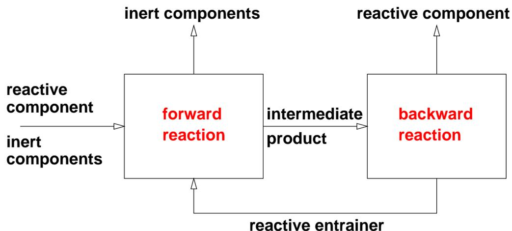
**Fig. 19:** Simplified flowsheet of the proposed reactive separation process.
