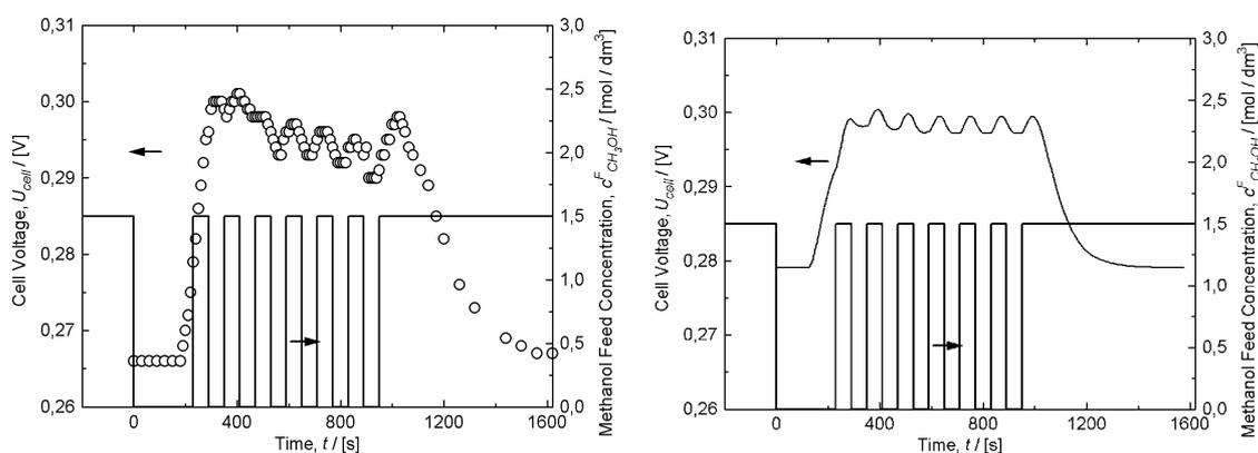
**Fig. 30:** Cell voltage response to periodically pulsed methanol feed concentration: experimental data (top) and simulation (bottom) at  $T=70^{\circ}\text{C}$ ,  $c_{\text{FCH3OH}}=1.5 \text{ mol/l}$ ,  $V_{\text{F}}=1.36 \text{ ml/min}$ ,  $p_{\text{a}}=0.1 \text{ MPa}$ ,  $p_{\text{c}}=0.3 \text{ MPa}$  [18].
