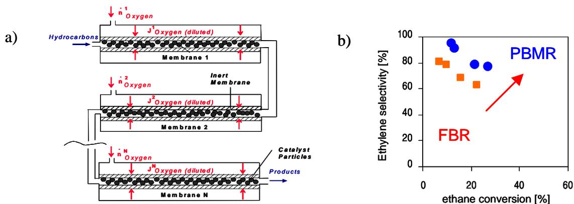
**Fig. 61:** a) Experimental setup of a packed bed membrane reactor (PBMR), b) Performance of fixed bed reactor (FBR) and PBMR [33, 35].
