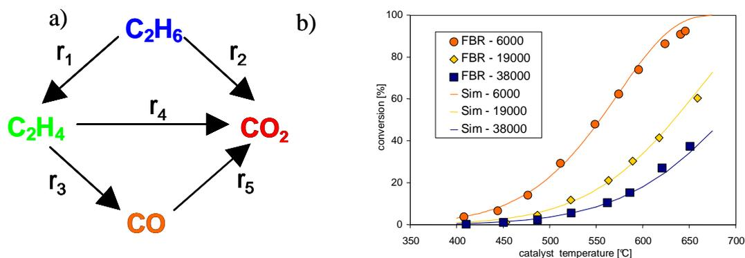
**Fig. 54:** Quantified reaction network of the oxidative dehydrogenation of ethane and predicted (Sim) versus measured conversions in a fixed-bed reactor (FBR) for several residence times (in  $\text{s}^{-1}$ ) [8, 9].
