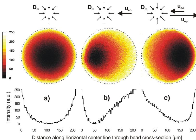
**Fig. 59:** Distribution of fluorescent molecules in a porous glass bead during intraparticle transport by diffusion (left) diffusion and electroosmosis (center) and diffusion, electroosmosis and electrophoresis (right) [26].
