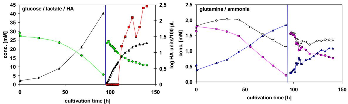
**Fig. 64:** Profiles of metabolites (left: glucose ●, lactate ▲ and HA ■; right: total glutamine ●, glutamine without chemical decomposition ○ and ammonium ▲) during growth of MDCK cells on microcarriers in a 5 L stirred bioreactor (left side of blue vertical line) and during influenza virus production after medium exchange (right side of blue line); biochemistry analyzer YSI 7100 (YSI, Yellow Springs, USA) and Vitros DT60-II (Ortho Clinical Diagnostics, Neckargemünd, Germany).
