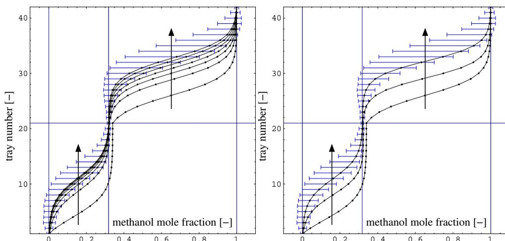
**Fig. 45:** Start-up of a distillation column: open-loop (left,  $\Delta = 5h$ ), closed-loop (right,  $\Delta = 10 \text{ min}$ ).
