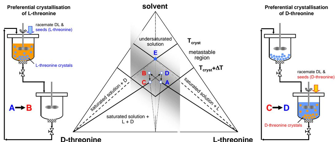
**Fig. 56:** Principle of the preferential crystallization and a possible quasi-continuous operation mode.
