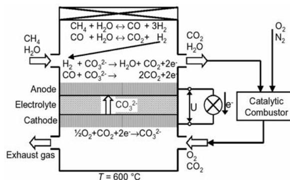
**Fig. 34:** Working principle of Molten Carbonate Fuel Cell with direct internal reforming. As an important basis for the experimental part of this research project, a 300 kW MCFC
