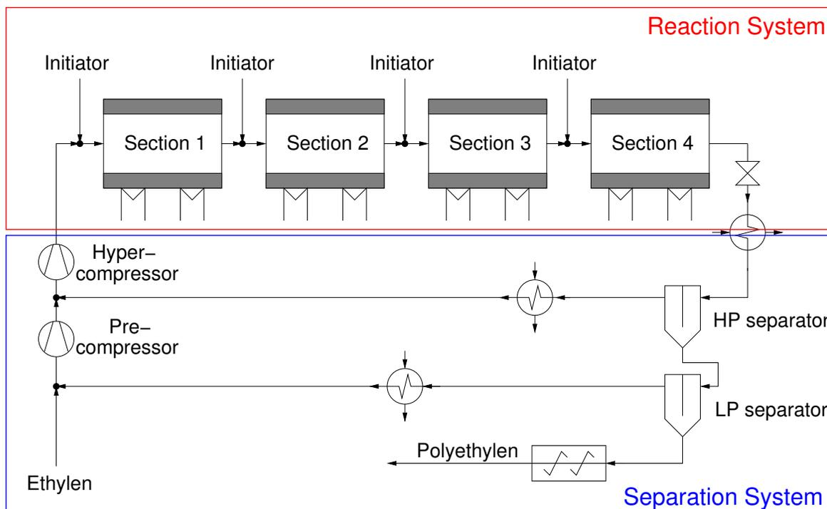
**Fig. 21:** Simplified flowsheet of an industrial plant for the production of low density polyethylene.
