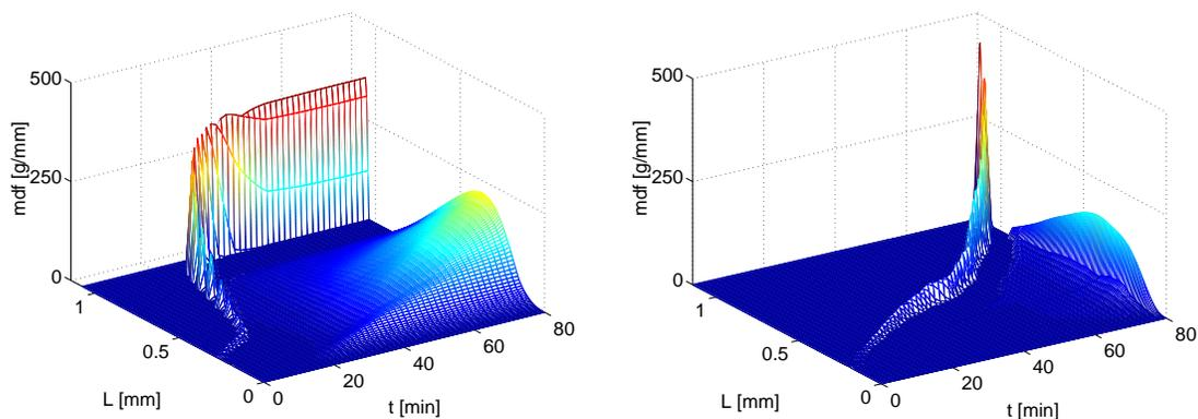
**Fig. 44:** Temporal evolution of CSD in a batch crystalliser: linear cooling policy (left), optimal cooling policy (right).
