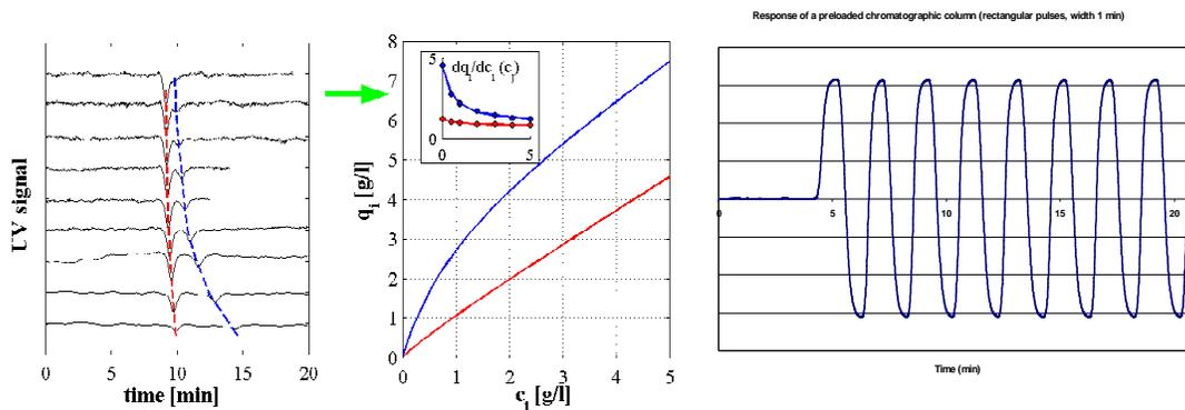
**Fig. 53:** Left: Determination of isotherm parameters by perturbation method. The retention times of small perturbations applied to a column equilibrated on different concentration levels can be related to the local derivatives of an isotherm model (centre, inset) [5, 6]. Right: Primary data for a frequency response analysis of a chromatographic column [7].
