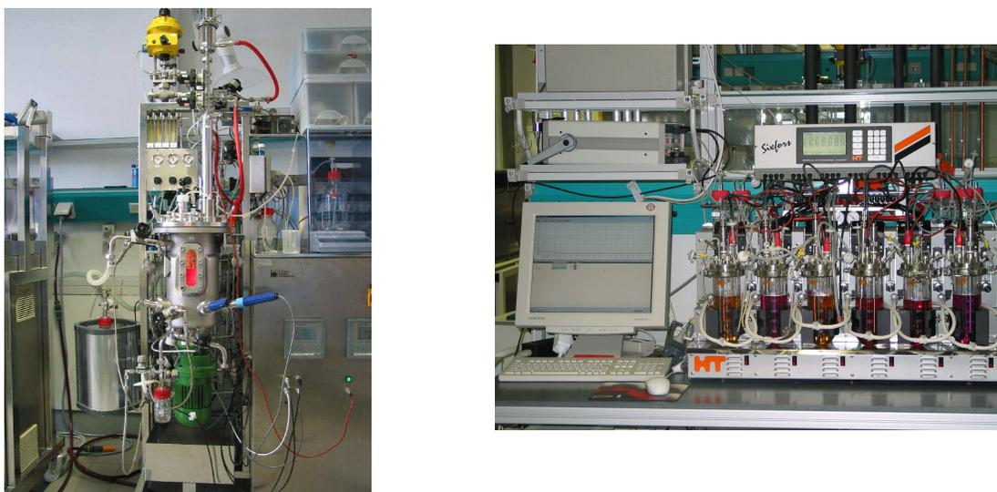
**Fig. 63:** Two possibilities for controlled cultivation using microcarrier systems in our lab (5 L bioreactor (B. Braun Biotech, Melsungen, Germany) and 6 parallel reactors of 0.5 L (Infors, Basel, Switzerland).
