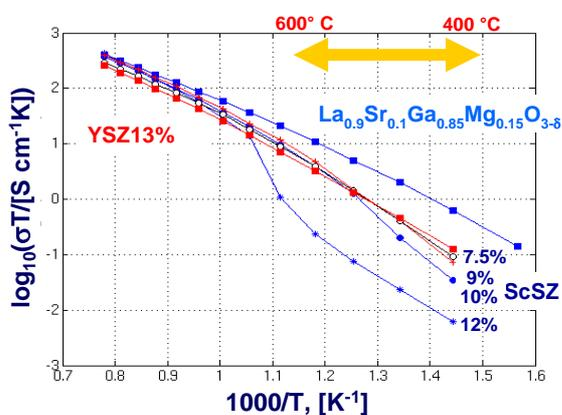
**Fig. 37:** Ionic conductivities of different membrane materials in dependence on temperature [30].
