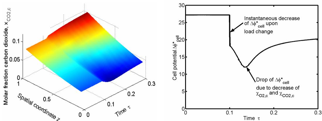
**Fig. 35:** Step responses of MCFC state variables to current load change (dimensionless quantities). Left:  $CO_2$  concentration along the cathode channel; right: overall cell potential [25].
