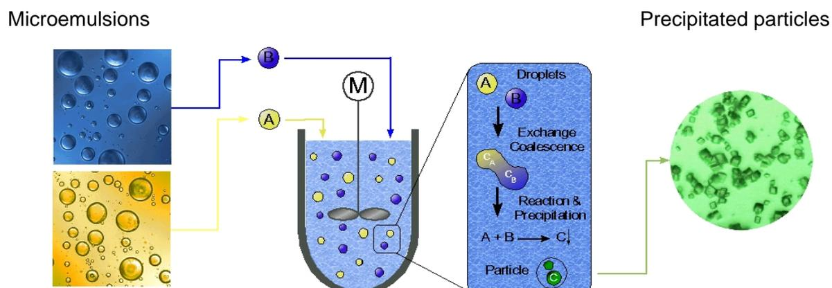
**Fig. 39:** Formation of solid particles by precipitation in microemulsions: principle of the process.
