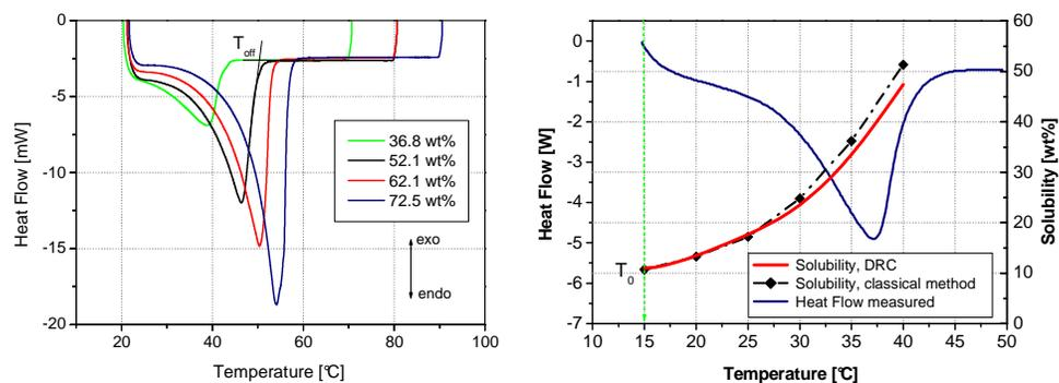
**Fig. 51:** Left: Differential Scanning Calorimetry (DSC) curves for solutions of different concentration of a pharmaceutical intermediate in acetonitrile (DSC 111/Setaram, 68-78 mg sample mass, heating rate 1 K/min). Right: Determination of the solubility curve from a single calorimetric experiment (reaction calorimeter DRC/Setaram, 40 wt% rac. mandelic acid in water, total sample mass 70 g, heating rate 0.5 K/min) [1, 3].
