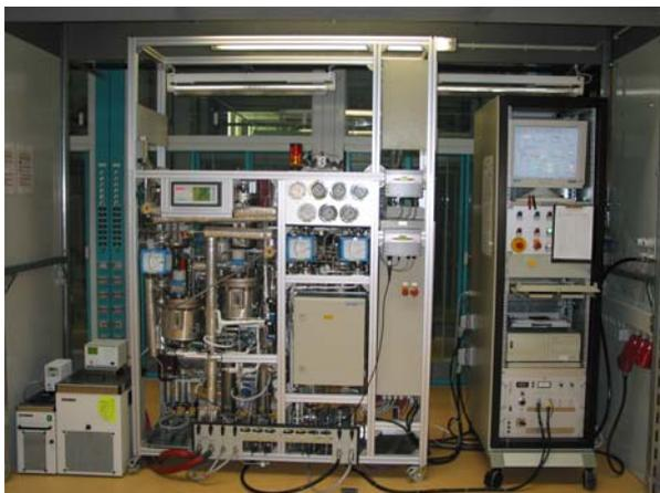
**Fig. 28:** DMFC miniplant installed in technical hall.
