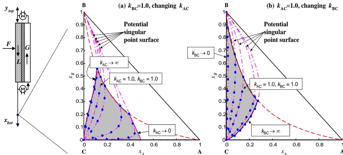
**Fig. 27** Feasible bottom product regions (shadowed) of a membrane reactor at different mass transfer coefficients in the membrane for the reaction  $A + B \rightleftharpoons C$  (dashed: chem. Equilibrium line) [12].
