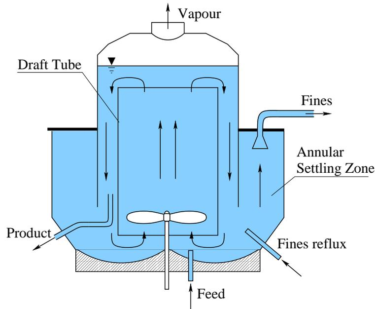
**Fig. 41:** Continuous crystalliser.
