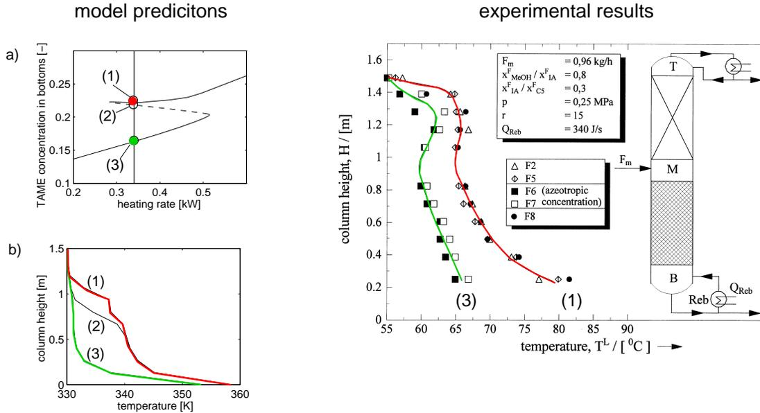
**Fig. 18:** Multiple steady states for the production of fuel ether TAME by reactive distillation.
