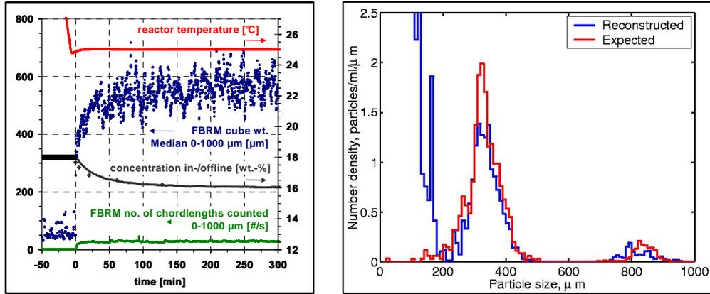
**Fig. 52:** Left: Isothermal crystal growth experiment for determination of growth kinetic parameters, time = 0 min: seed crystals of a specific size fraction are added to a supersaturated solution, FBRM no. of chordlengths counted: confirms pure growth without spontaneous nucleation, concentration (offline): density measurements, concentration (inline): acoustically determined. Right: Comparison of expected and reconstructed particle size distribution based on FBRM measurements [4].
