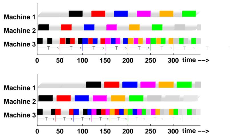
**Fig. 47:** Examples for cyclic operating scheme (Gantt charts). Individual batches are shown in different colors.
