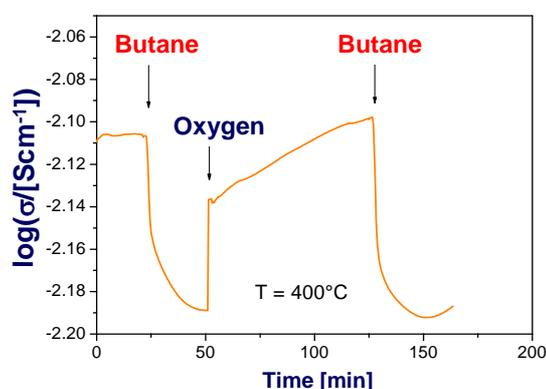
**Fig. 38:** Change of total conductivity of VPO catalyst by alternating butane and oxygen feed [30].
