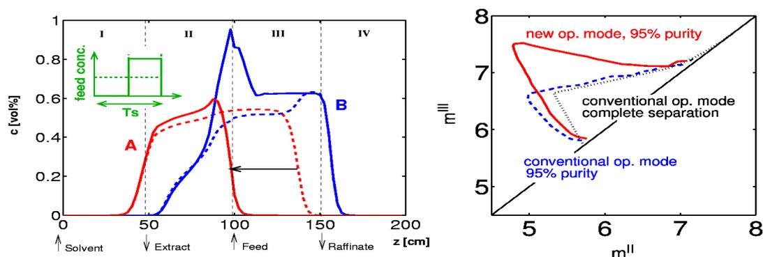
**Fig. 58:** Left: Effect of a non-constant feed concentration on the internal concentration profiles in a SMB unit. Right: Corresponding changes of the area of possible operation parameters (“separation region”) [18 – 21].
