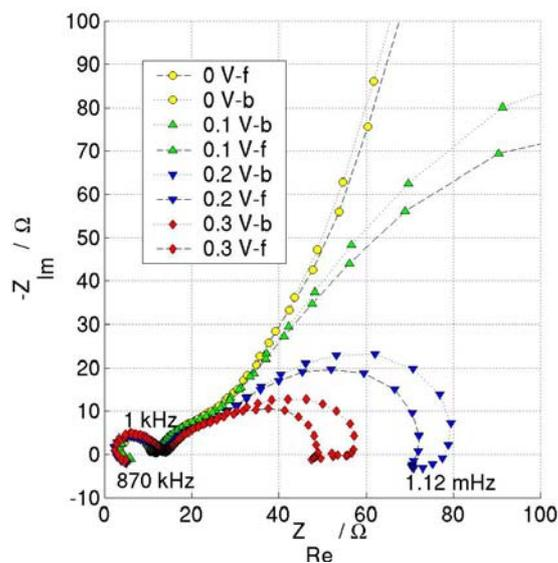
**Fig. 32** Impedance spectra for electrochemical methanol oxidation at carbon supported Pt/Ru electrodes [21]. (f = increasing, b = decreasing frequencies)
