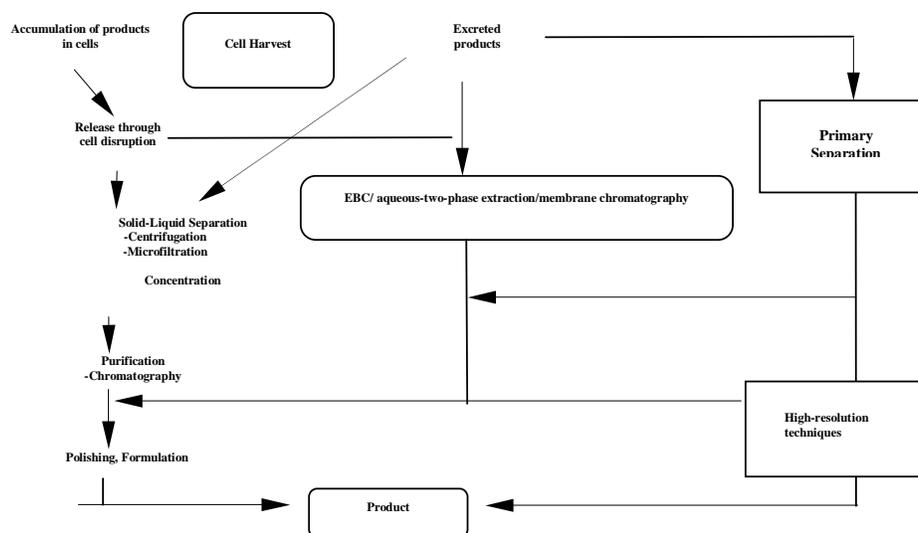
**Fig. 72:** Overview on downstream processing methods.
