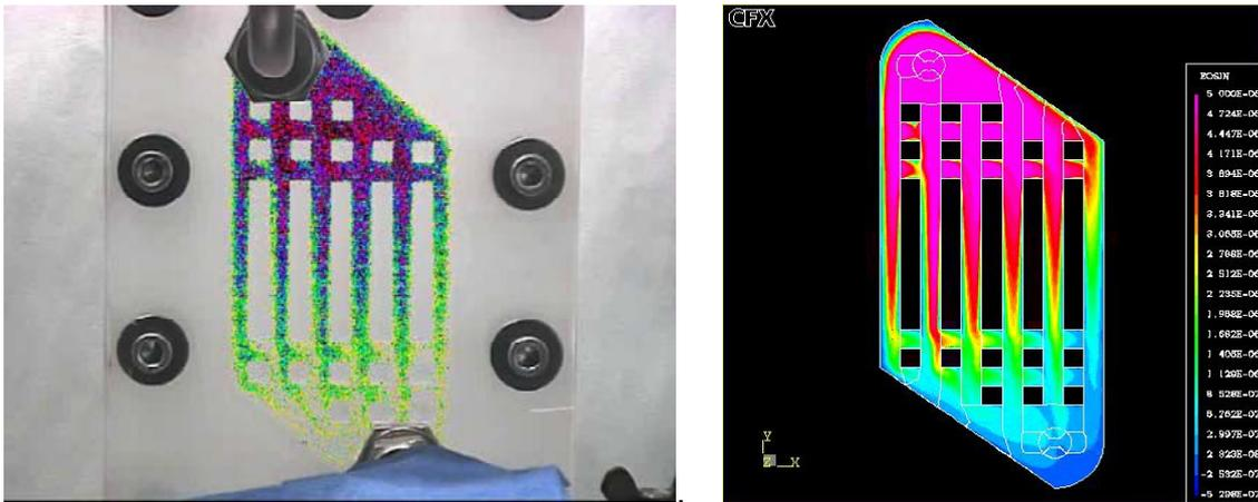
**Fig. 33:** Snapshot of the dynamic tracer mixing process in the liquid filled anode manifold of a DMFC, left: experimental tracer visualisation, right: 3D CFD simulation carried out with CFX [24].
