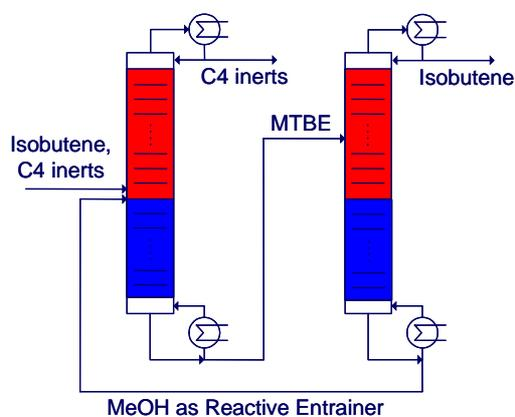
**Fig. 25:** Coupled reactive distillation columns for the separation of C4 fractions [7].
