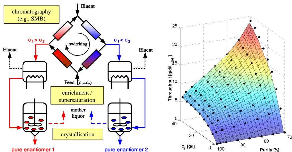
**Fig. 60:** Example for two coupled separation processes. A racemic feed is partially resolved by SMB-chromatography and then split into the pure enantiomers by subsequent enantioselective crystallization (left). Numerical simulation for a pharmaceutical compound reveal the possibility of substantially increased productivity of the chromatographic step (right) [28, 29].
